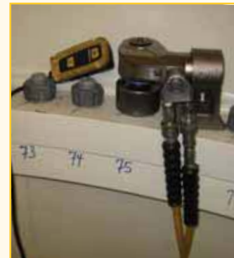
▲ S3000 used to connect wind tower segments
